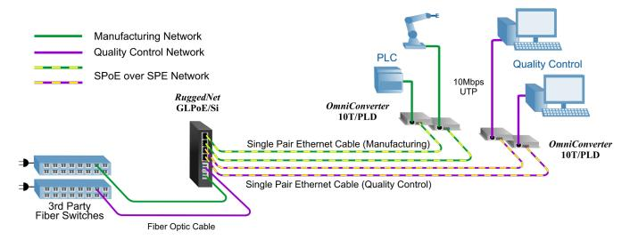
The RuggedNet switch, PLC, robot and computers will require an external power source.
