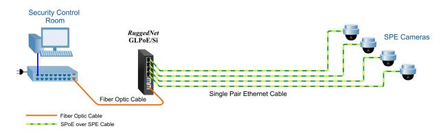
The RuggedNet switch will require an external power source.
