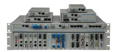
*iConverter* 4Tx modules are hot-swappable and can be mounted in a 19-Module (2U high) or 5-Module (1U high) rackmountable chassis (19-inch or 23-inch) with any combination of redundant AC, 24VDC or 48VDC power supplies. They can also be mounted in a 2-Module AC or 18 to 60VDC powered chassis, or in a 1-Module AC/DC powered chassis.
