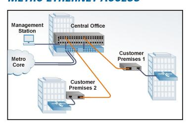
At the Central Office, the GX/TM2 plug-in module is installed in a managed *iConverter* 19-Module chassis for high-density fiber distribution from UTP switch equipment. At Customer Premises 1 and 2, GX/TM2 standalone NIDs provide a fiber uplink to a single copper port for intelligent demarcation of Ethernet services.
