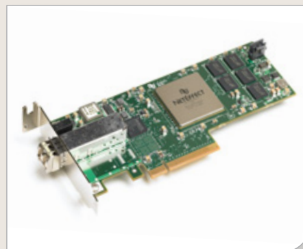
NetEffect Ethernet Server Cluster Adapter SFP+ SFP+ SR (E10G81GFSR), DA (E10G81GP) Single port SR optical media or pluggable
