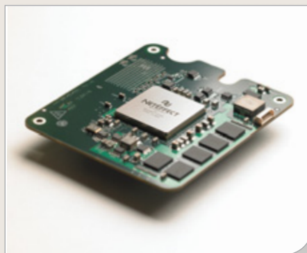
NetEffect Ethernet Mezzanine Adapter for the HP BladeSystem c-Class (K10G82GTKX4H) Dual port Type I form factor
