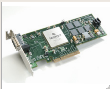
NetEffect Ethernet Server Cluster Adapter CX4 (E10G81GTCX4) Single port CX4 or Powered CX4
