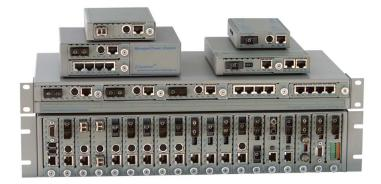
*iConverter* 4Tx modules are hot-swappable and can be mounted in a 19-Module (2U high) or 5-Module (1U high) rack-mountable chassis (19-inch or 23-inch) with any combination of redundant AC, 24VDC or 48VDC power supplies. They can also be mounted in a 2-Module AC or 18 to 60VDC powered chassis, or in a 1-Module AC/DC powered chassis.
