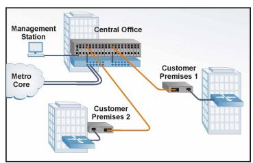
At the Central Office, the GX/TM2 plug-in module is installed in a managed *iConverter* 19-Module chassis for high-density fiber distribution from UTP switch equipment. At Customer Premises 1 and 2, GX/TM2 standalone NIDs provide a fiber uplink to a single copper port for intelligent demarcation of Ethernet services.
