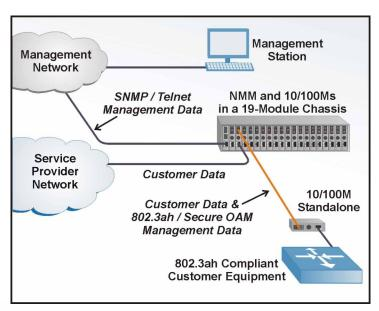
by the *iConverter* Network Management Module (NMM) in the 19-Module Chassis at the Central Office.
